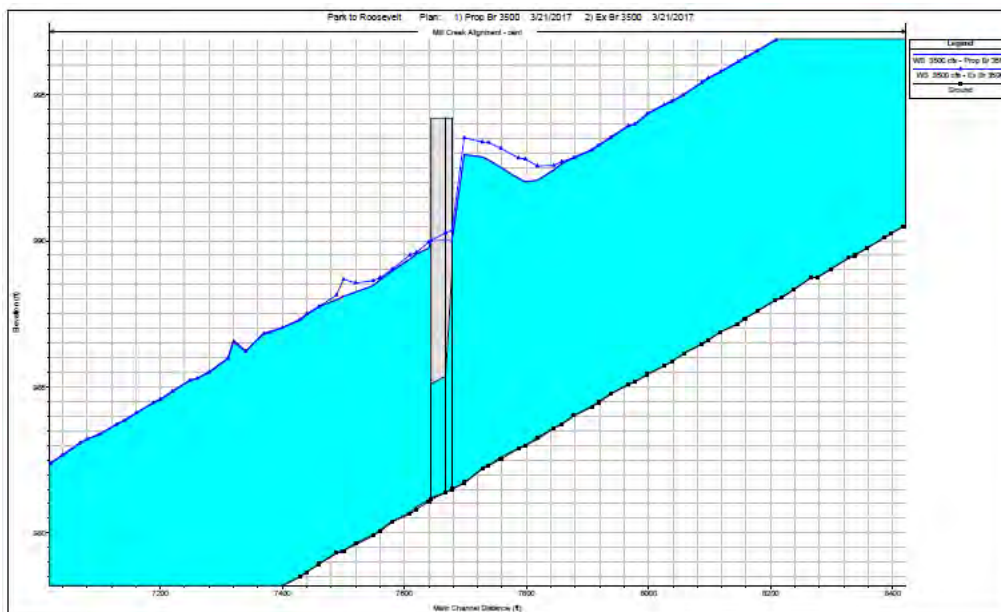
Figure 9 – Existing versus proposed water surface elevations from STA 7460 to 7847 (Merriam Bridge) at 3500 cfs. The blue line with triangles is the existing condition.
