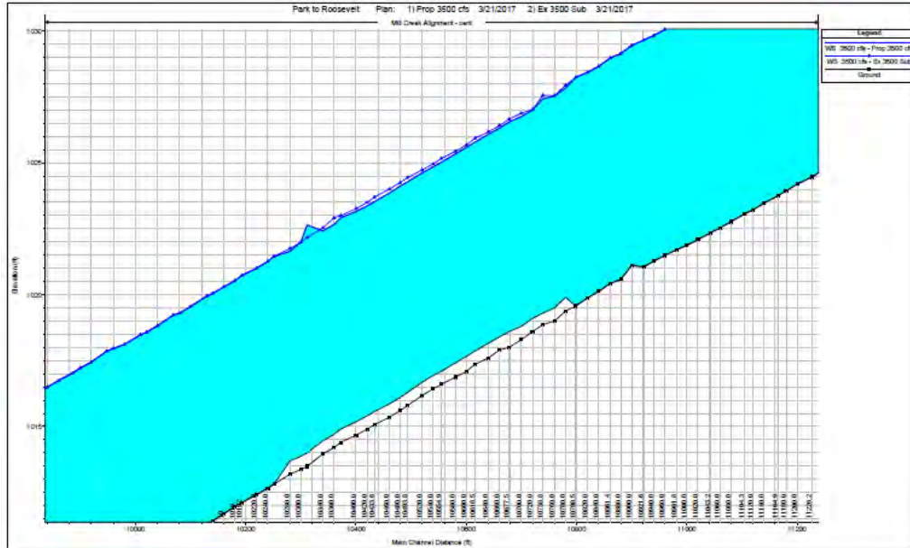
Figure 10 - Existing versus proposed water surface elevations from STA 10280 to 10780 at 3500 cfs. The blue line with triangles is the existing condition.
