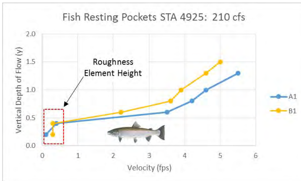
Figure 25 - Fish resting pocket velocities at Point 1, immediately downstream of the roughness element. The dashed red box is representative of the height of the roughness element.
