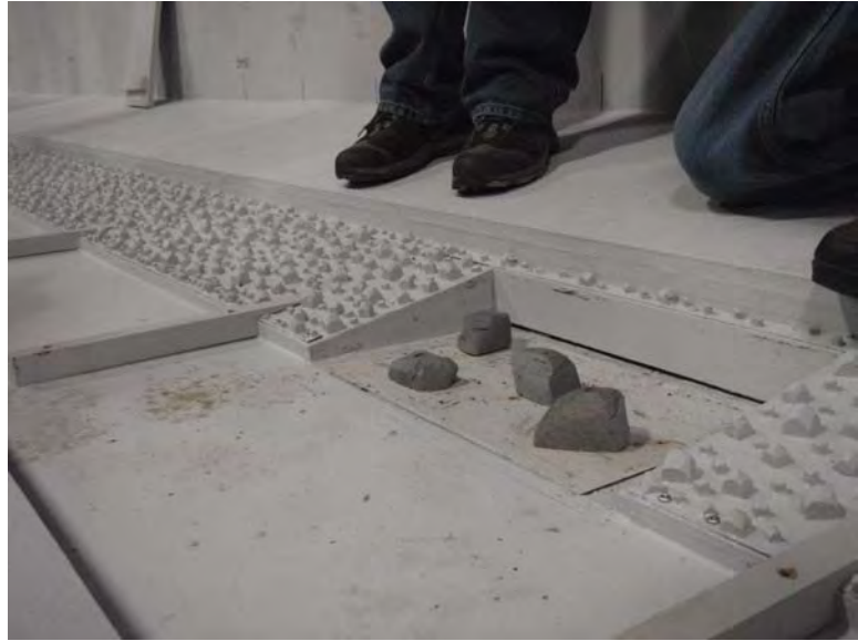
Figure 3 - Mill Creek 1:8 Physical Model Reach Type 3. View upstream showing resting pool with cover rocks, baffles and roughened channel.
