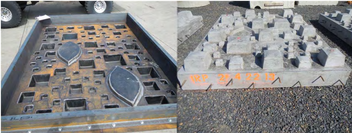
Figure 7 - Left Photo is the Steel Form Flipped Upside down, and the Right Photo is the Final Poured Panel. The Overall Roughness Height, Density and Spacing within the Values Used in the Physical Model Study.
