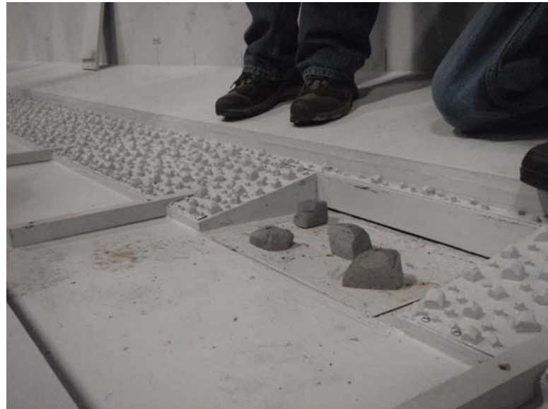
Figure 4 - Mill Creek 1:8 Physical Model Reach Type 3. View upstream showing resting pool with cover rocks, baffles and roughened channel.
