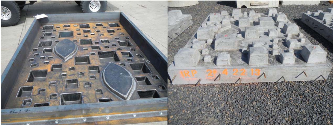
Figure 15 - Left Photo is the Steel Form Flipped Upside down, and the Right Photo is the Final Poured Form. The Overall Roughness Height, Density and Spacing within the Values Used in the Physical Model Study.
