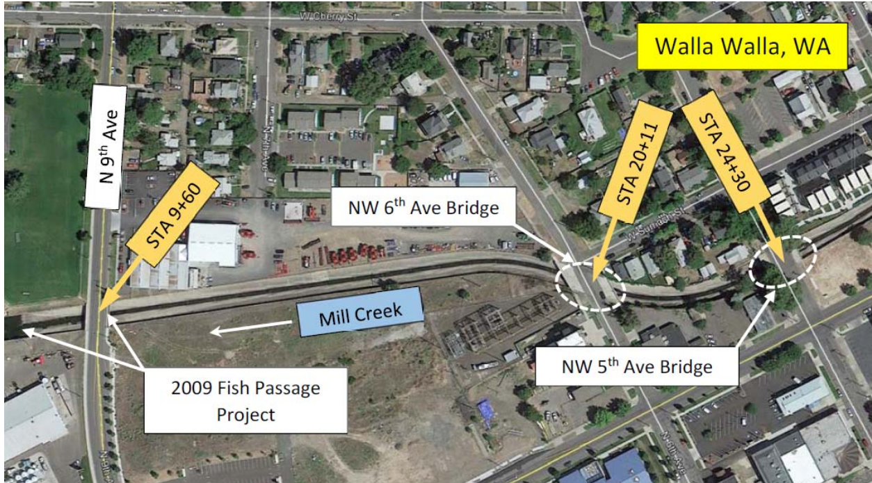
Figure 2 – Project site map. Mill Creek flow is from right to left. The downstream end of the concrete flume is STA 7+05. STA 0+00 is the Union Pacific Railroad.
