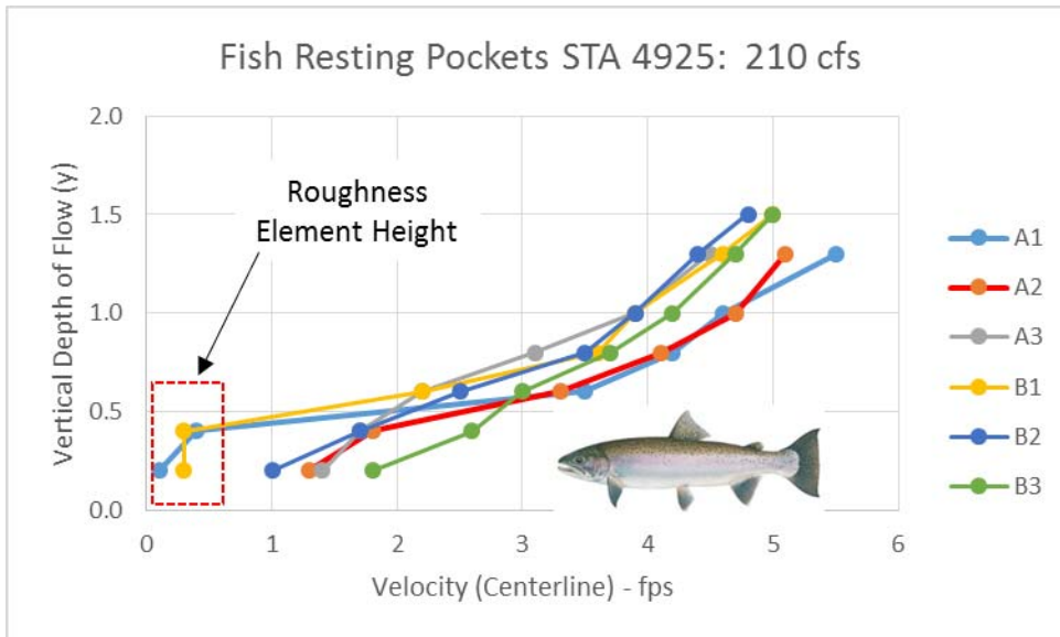
Figure 35 – Combination of Fish Resting Pocket velocities for all measurements.
