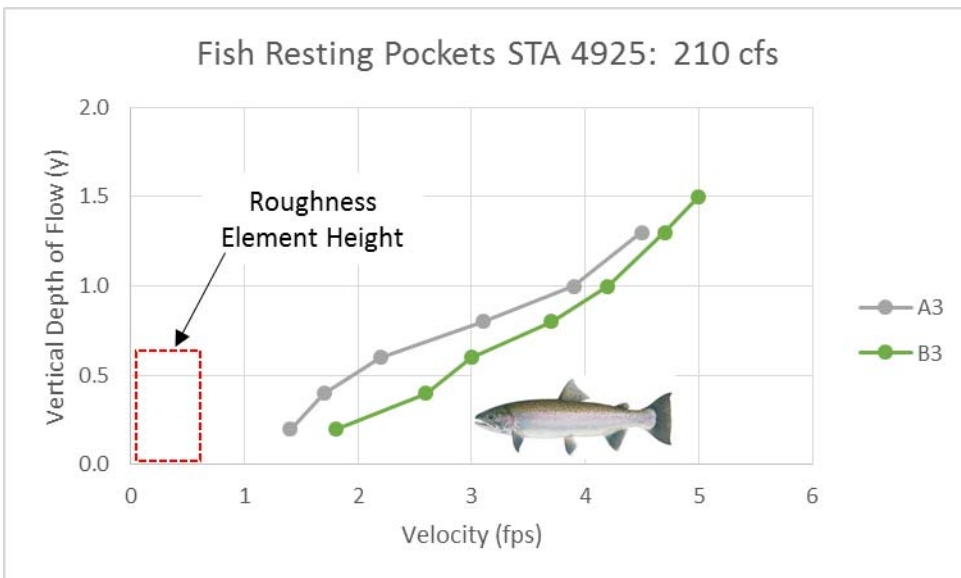
Figure 34 - Fish Resting Pocket velocities at Point 3 (downstream end of the resting pocket). The dashed red box is representative of the height of the roughness element.
