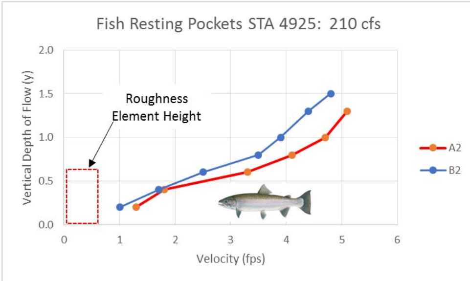
Figure 33 - Fish Resting Pocket velocities at Point 2 (center of the resting pocket). The dashed red box is representative of the height of the roughness element.
