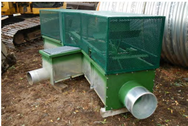
Water enters the screen to the rear of this view. Fish leave through the pipe on the left, while fish-free water flows out the pipe closest to the viewer. A paddlewheel inside the unit propels a brush that cleans the screen.
