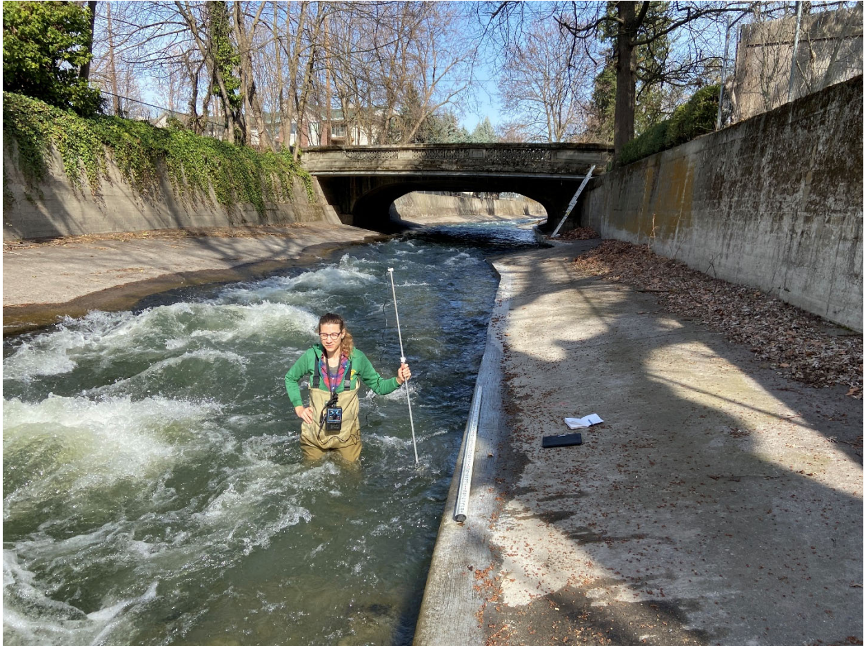
Photo 11 –Resting Pool 5 just downstream of Merriam Street. Velocities on the left side of the photo are 6 to 8 fps, but only 1 to 2 fps in the pool.
